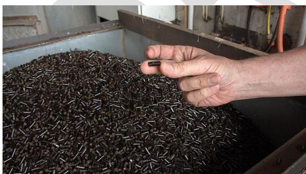
Figure 20: Pellets from Digestate (picture credits: IBBK Fachgruppe Biogas GmbH)
