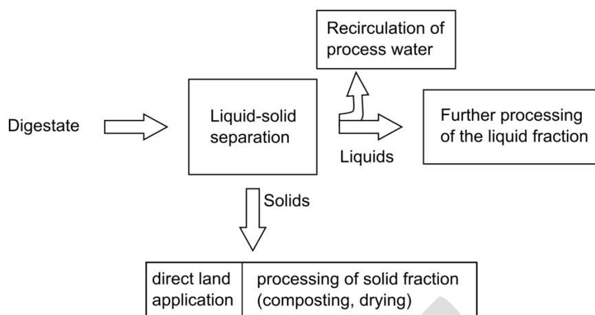
Figure 18: Basic processes of digestate upgrading (Fuchs & Drosig, 2010)
